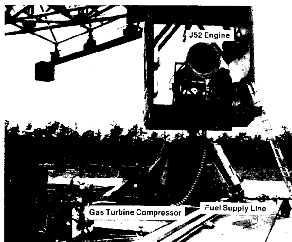
Fig. 7 J52 engine installed in gyro rig.
